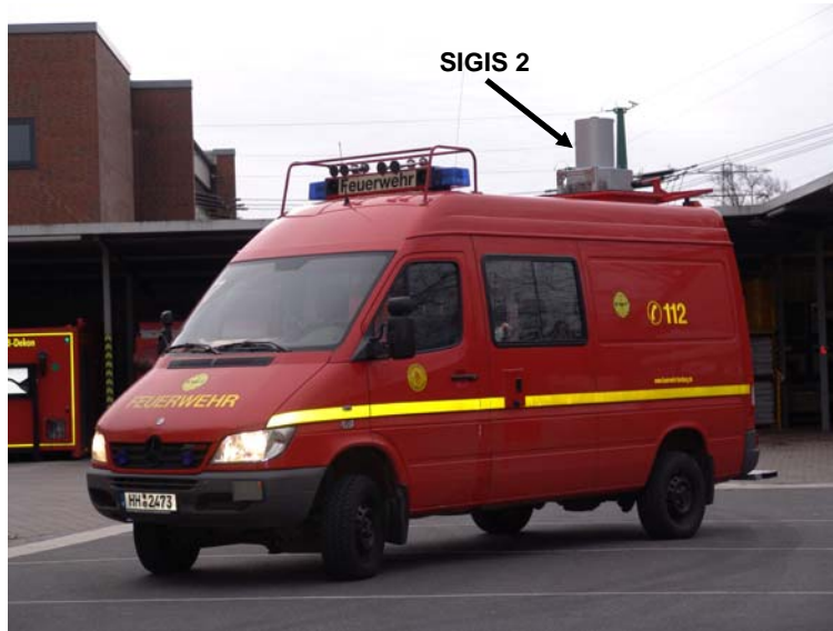
Fig. 2: SIGIS 2 mounted in a vehicle of the fire brigade of Hamburg (Photo: T. Lübke-Horn).
